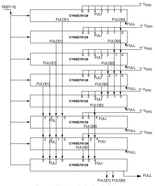
Figure 11-3. FULL Generation in a Cascaded Table
