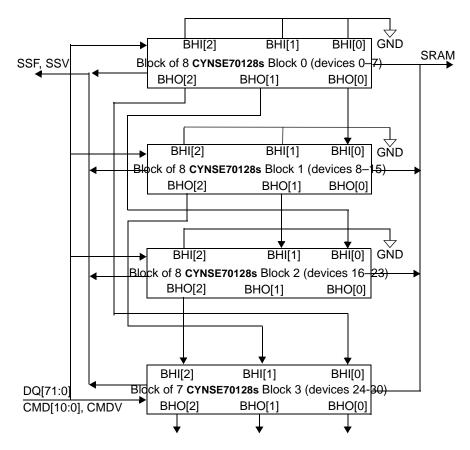
Figure 11-2. Depth-Cascading Four Blocks
