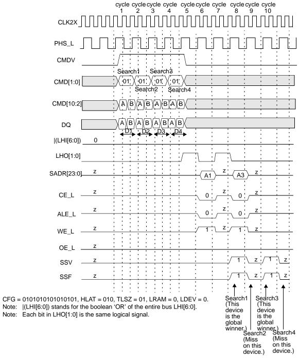
Figure 10-31. Timing Diagram for 144-bit Search Device Number 0
