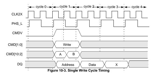
The following is the Write operation sequence, and *Table* shows the Write address format for the data array, the mask array, or the single-Write SRAM. *Table 10-8* shows the Write address format for the internal registers.
