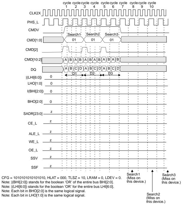
Figure 10-60. Timing Diagram for Each Device Above the Winning Device in Block Number 1
