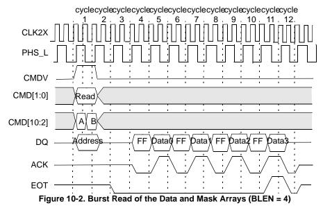
The Read operation lasts 4 + 2n CLK cycles (where n is the number of accesses in the burst specified by the BLEN field of the RBURREG) in the sequence shown below. This operation assumes that the host ASIC has programmed the RBURREG with the starting address (ADR) and the length of the transfer (BLEN) before initiating the burst Read command.
