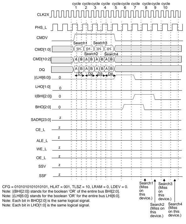
Figure 10-46. Timing Diagram for Devices Below the Winning Device in Block Number 3 Except Device 30 (the Last Device)
