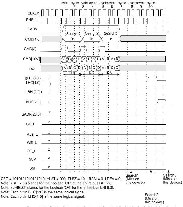
Figure 10-62. Timing Diagram for Devices Below the Winning Device in Block Number 1
