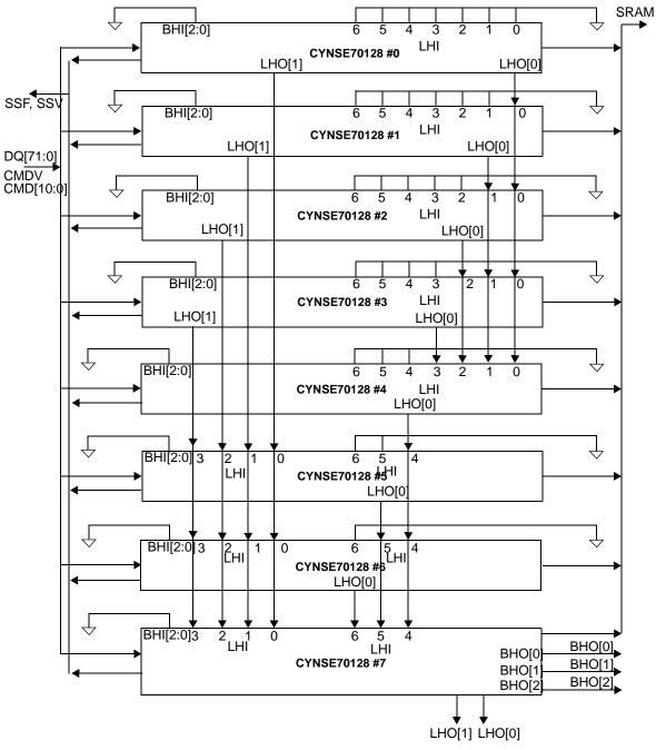
Figure 10-52. Hardware Diagram for a Table with Eight Devices
