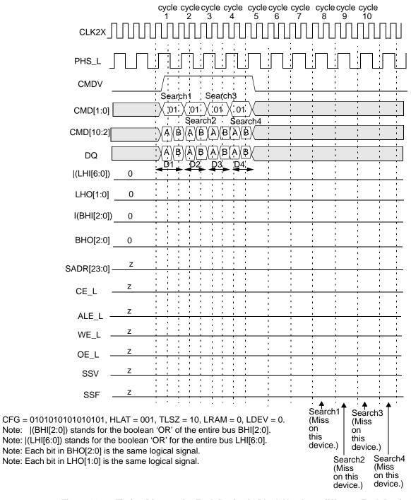
Figure 10-37. Timing Diagram for Each Device in Block Number 0 (Miss on Each Device)
