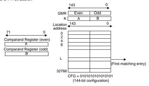
Figure 10-29. x144 Table with One Device
