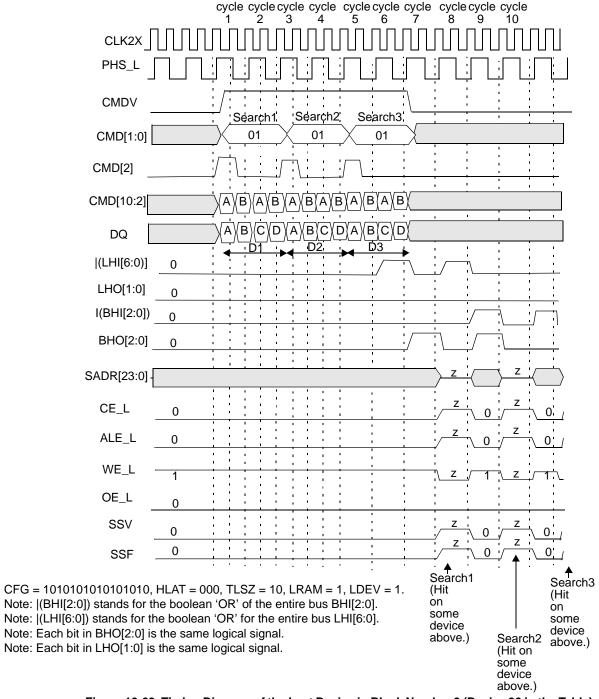
Figure 10-69. Timing Diagram of the Last Device in Block Number 3 (Device 30 in the Table)
