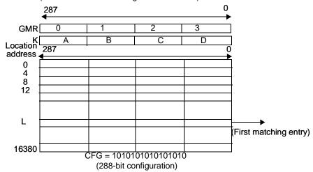
Figure 10-51. x288 Table with One Device
