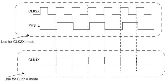
Figure 5-3. CYNSE70128 Clocks for All Timing Diagrams
