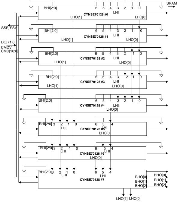
Figure 12-2. Table of a Block of Eight Devices
