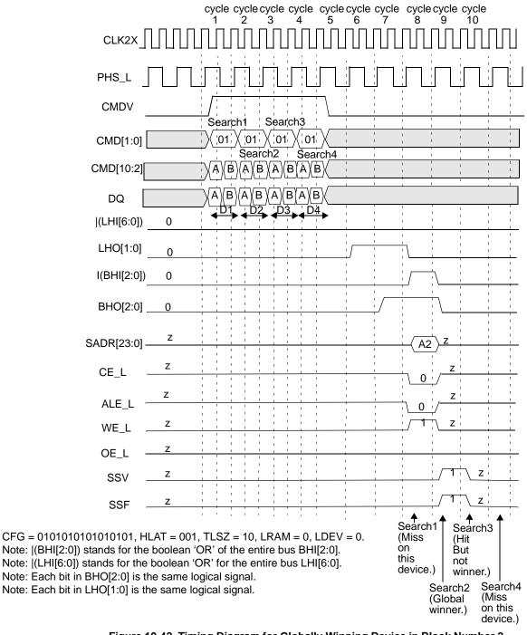
Figure 10-42. Timing Diagram for Globally Winning Device in Block Number 2
