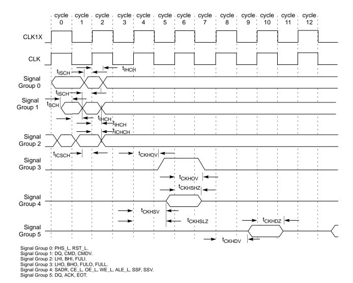
Figure 17-5. AC Timing Waveforms with CLK1X
