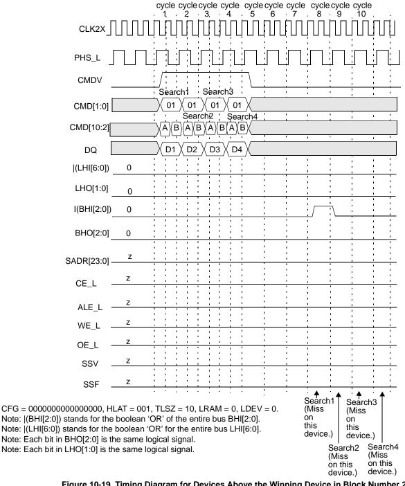
Figure 10-19. Timing Diagram for Devices Above the Winning Device in Block Number 2
