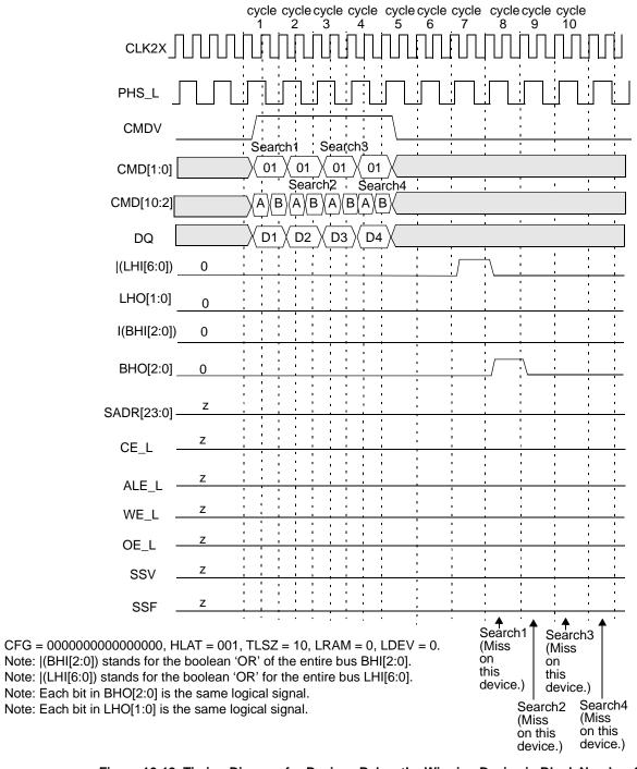
Figure 10-18. Timing Diagram for Devices Below the Winning Device in Block Number 1
