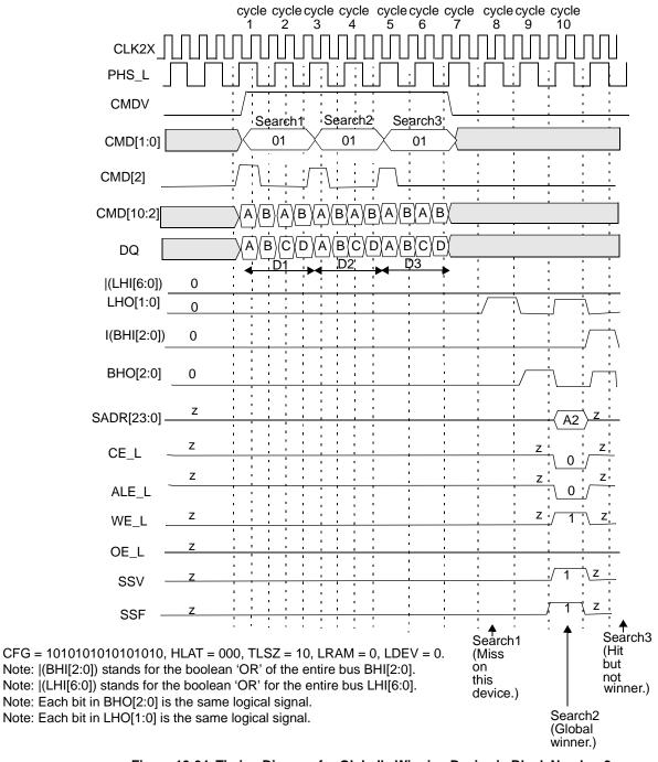
Figure 10-64. Timing Diagram for Globally Winning Device in Block Number 2
