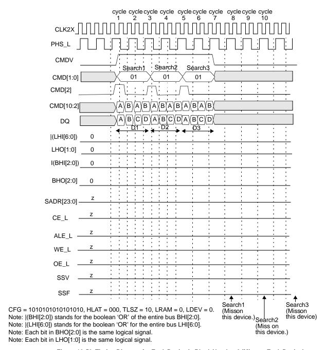
Figure 10-59. Timing Diagram for Each Device in Block Number 0 (Miss on Each Device)
