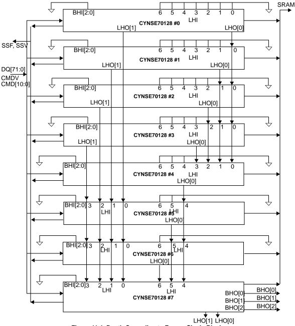
Figure 11-1. Depth-Cascading to Form a Single Block
