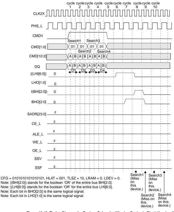
Figure 10-43. Timing Diagram for Devices Below the Winning Device in Block Number 2
