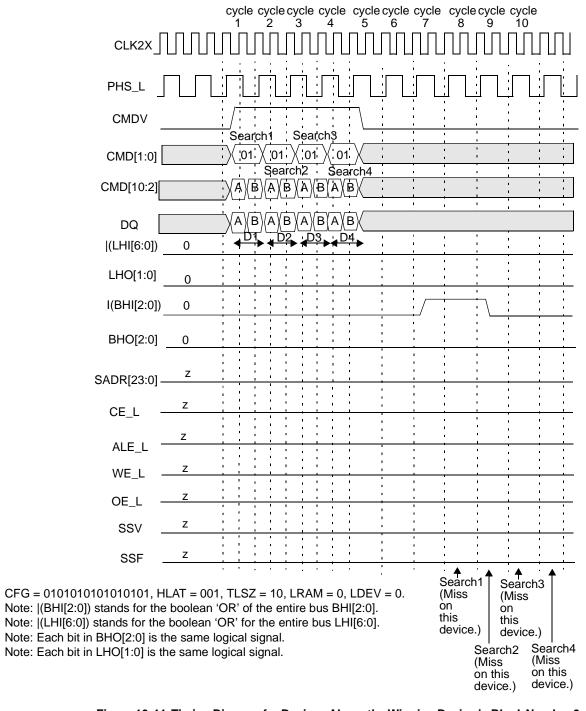
Figure 10-44. Timing Diagram for Devices Above the Winning Device in Block Number 3
