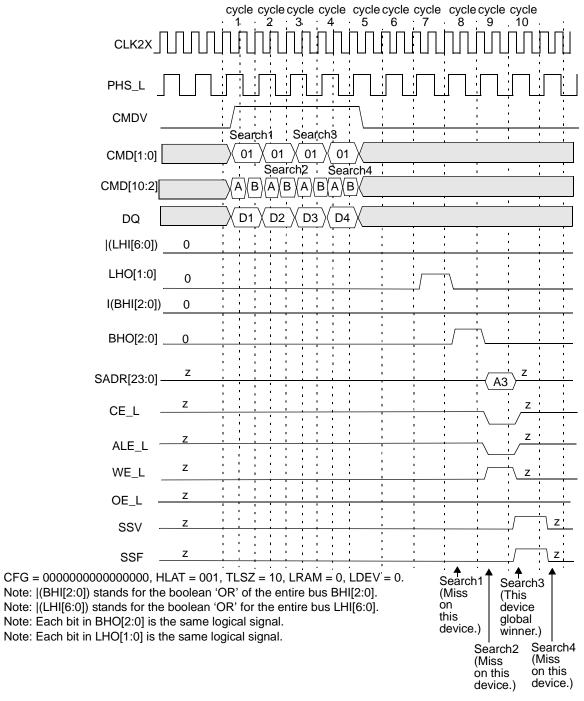
Figure 10-17. Timing Diagram for Globally Winning Device in Block Number 1
