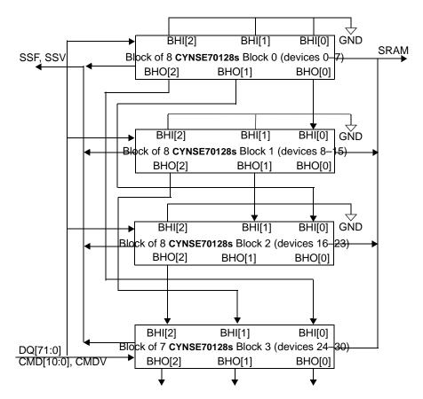
Figure 12-5. Table of 31 Devices Made of Four Blocks
