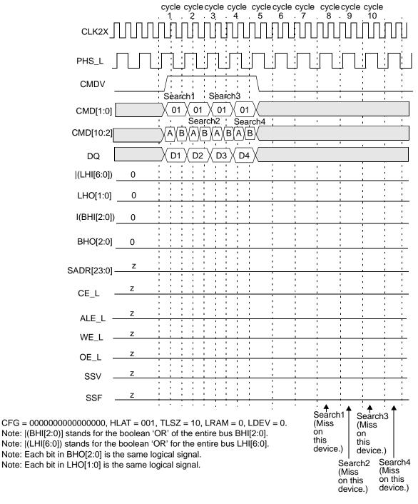
Figure 10-16. Timing Diagram for Each Device Above the Winning Device in Block Number 1
