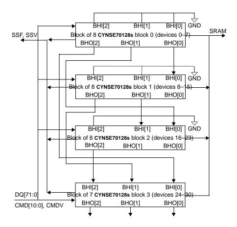
Figure 10-57. Hardware Diagram for a Table with 31 Devices
