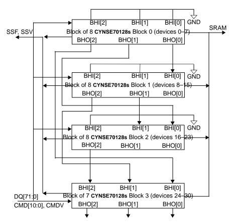
Figure 12-12. Table of 31 Devices (Four Blocks)
