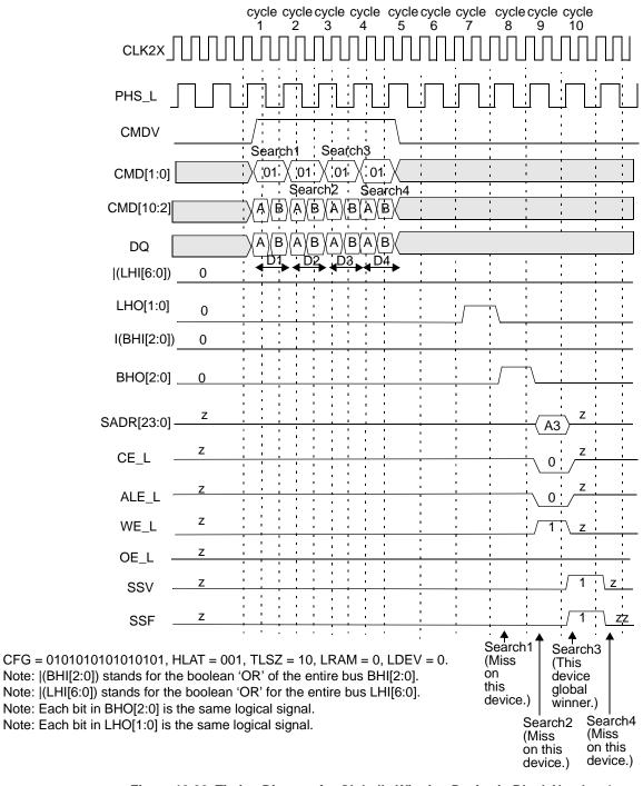
Figure 10-39. Timing Diagram for Globally Winning Device in Block Number 1
