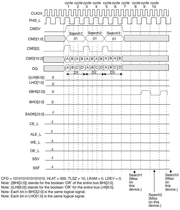
Figure 10-66. Timing Diagram for Devices Above the Winning Device in Block Number 3
