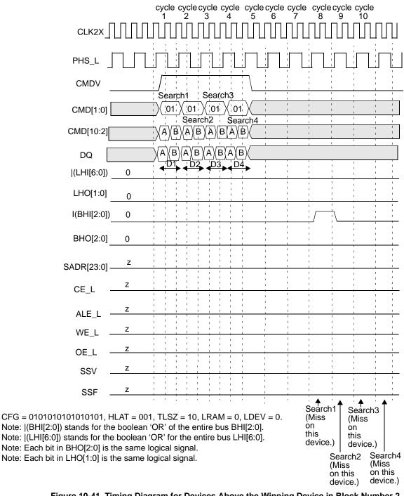
Figure 10-41. Timing Diagram for Devices Above the Winning Device in Block Number 2
