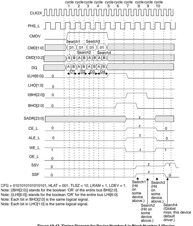
Figure 10-47. Timing Diagram for Device Number 6 in Block Number 3 (Device 30 in Depth-Cascaded Table)
