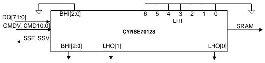
Figure 10-6. Hardware Diagram for a Table with One Device
