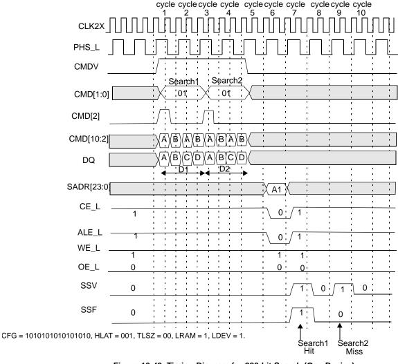
Figure 10-49. Timing Diagram for 288-bit Search (One Device)
