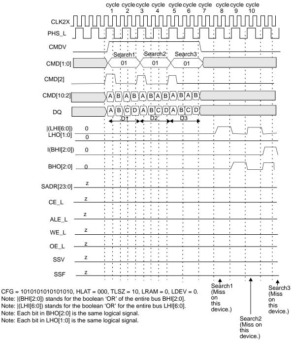
Figure 10-65. Timing Diagram for Devices Below the Winning Device in Block Number 2
