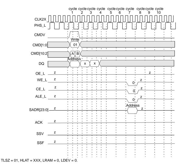
Figure 12-10. SRAM Write Through Device Number 0 in a Block of Eight Devices
