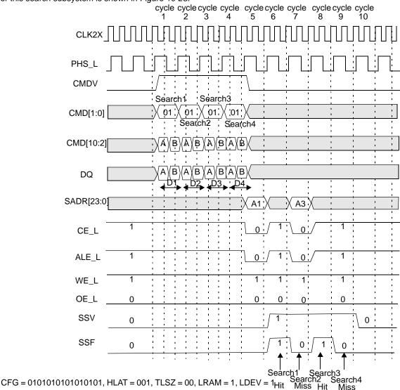
Figure 10-27. Timing Diagram for 144-bit Search (One Device)
