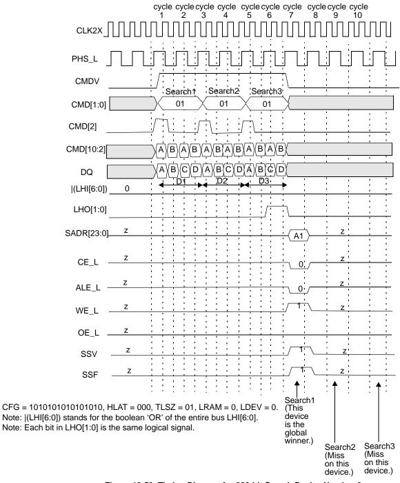
Figure 10-53. Timing Diagram for 288-bit Search Device Number 0
