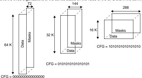
Figure 8-1. CYNSE70128 Database Width Configuration
