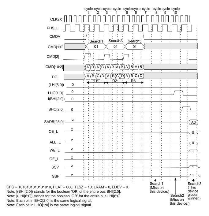
Figure 10-61. Timing Diagram for Globally Winning Device in Block Number 1
