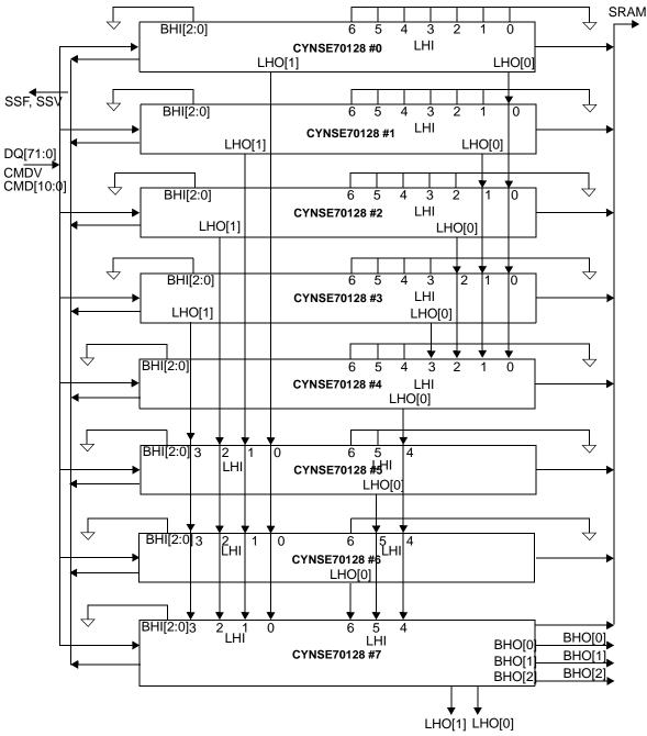
Figure 10-30. Hardware Diagram for a Table with Eight Devices
