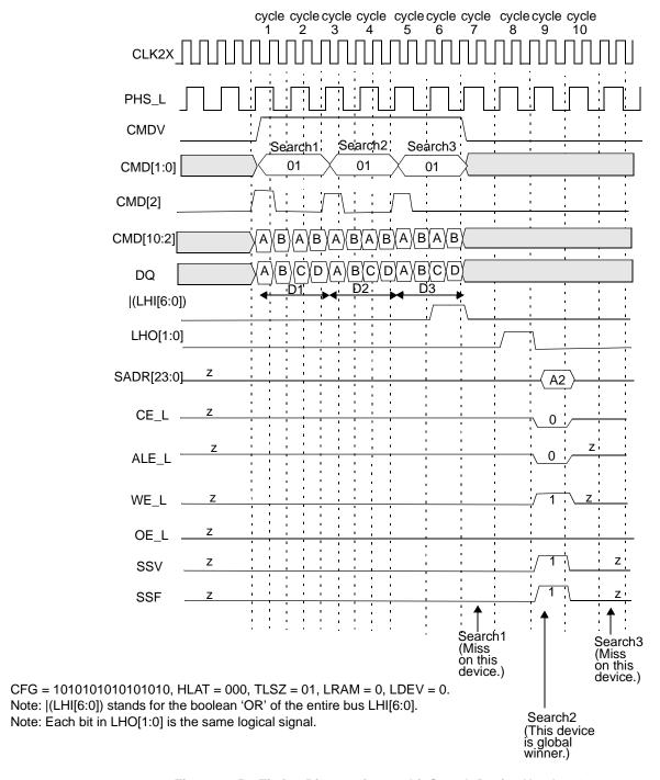
Figure 10-54. Timing Diagram for 288-bit Search Device Number 1
