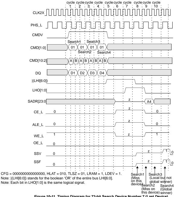
Figure 10-11. Timing Diagram for 72-bit Search Device Number 7 (Last Device)
