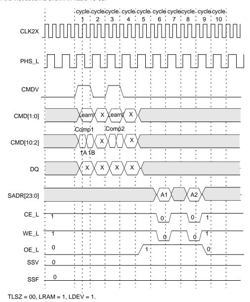
Figure 10-73. Timing Diagram of Learn (TLSZ = 00)
