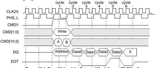
Figure 10-4. Burst Write of the Data and Mask Arrays (BLEN = 4)
