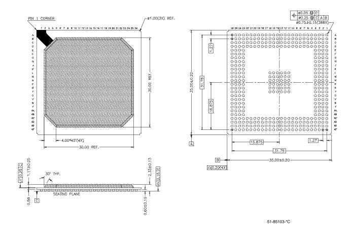
Figure 20-1. 388-lead Ball Grid Array (35 x 35 x 2.33 mm) BG388
