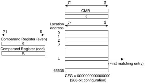
Figure 10-7. x72 Table with One Device
