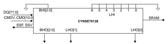
Figure 10-50. Hardware Diagram for a Table with One Device
