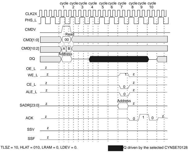
Figure 12-6. SRAM Read Through Device Number 0 in a Block of 31 Devices (Device Number 0 Timing)
