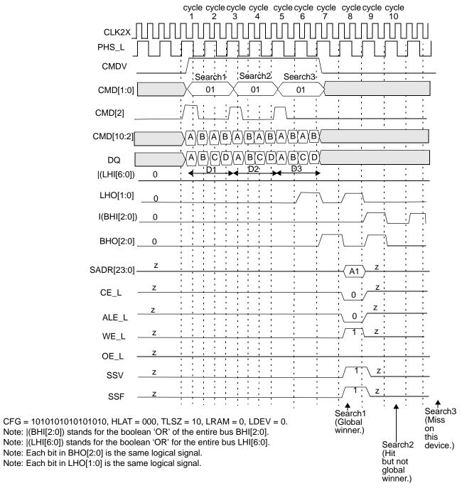
Figure 10-67. Timing Diagram for Globally Winning Device in Block Number 3
