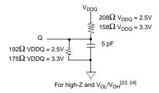
Figure 17-3. I/O Output Load Equivalent for CYNSE70128
