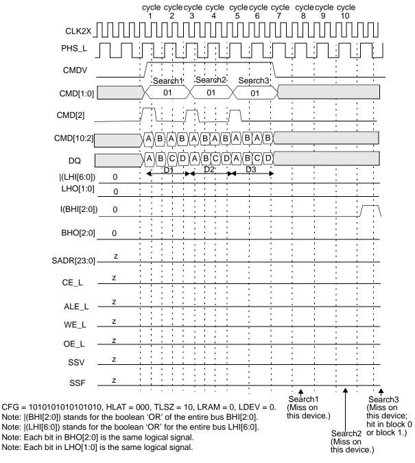
Figure 10-63. Timing Diagram for Devices Above the Winning Device in Block Number 2
