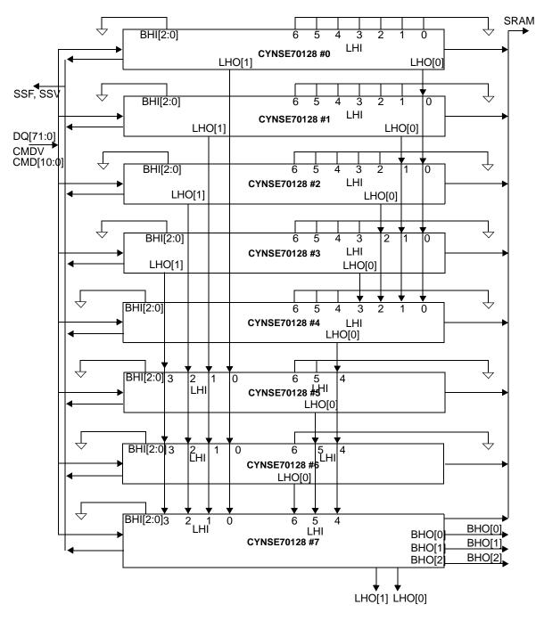
Figure 12-9. Table of a Block of Eight Devices
