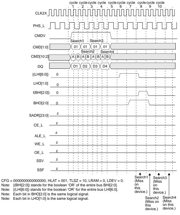
Figure 10-21. Timing Diagram for Devices Below the Winning Device in Block Number 2
