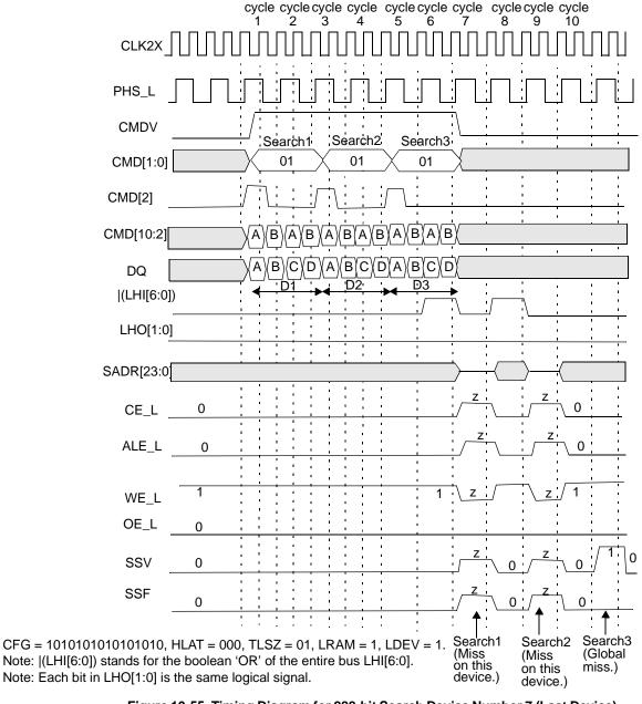
Figure 10-55. Timing Diagram for 288-bit Search Device Number 7 (Last Device)
