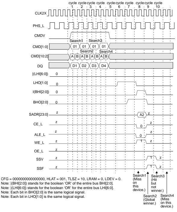
Figure 10-20. Timing Diagram for Globally Winning Device in Block Number 2
