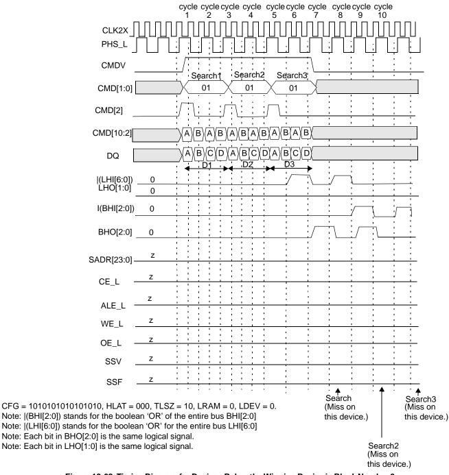
Figure 10-68. Timing Diagram for Devices Below the Winning Device in Block Number 3
