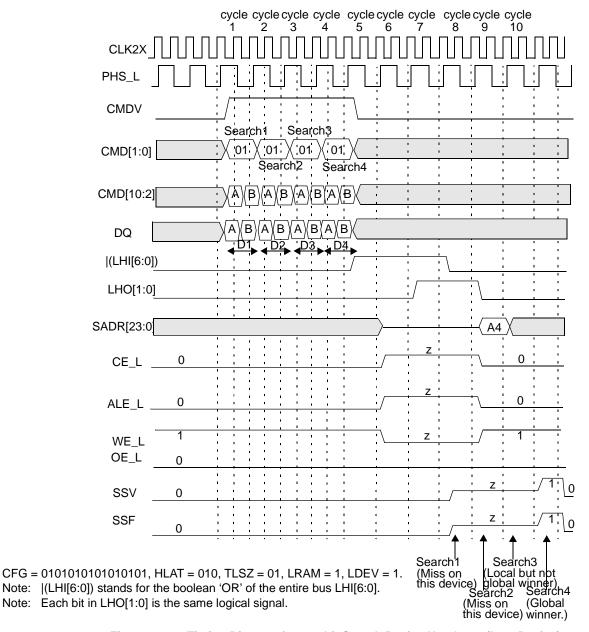
Figure 10-33. Timing Diagram for 144-bit Search Device Number 7 (Last Device)
